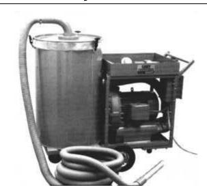
The **CARY** SuperVac System is designed to provide years of trouble-free service and continuous duty in industrial applications. Two versions are available, the stationary unit for central vacuum headers or limited are cleanups and the portable unit which employs a heavy-duty cart and can be moved to any location.
